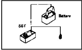
(1) Connect the SST to the battery. Connect the red clip of the SST to the battery positive (+) terminal and the black clip to the battery negetive (-) terminal.
