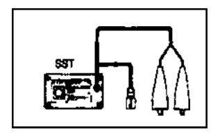
When deploying the airbag, always use the specified SST (SRS Airbag Deployment Tool). Perform the operation in a place away from electrical noise.
