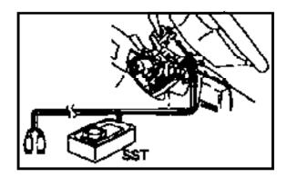
(3) Connect the SST connector to the airbag connector of the spiral cable.
